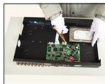
⑥ connect the power wire
